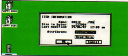
■ The "Show Info" dialogue box for a file. "Read-only" status means you can't write over or alter the data in the file – good protection if it's an important program
