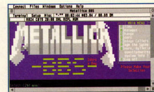
16-colour ANSI emulation is most often used for flashy graphics on PC bulletin boards, like the Metallica BBS shown here.
