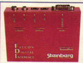
The FDI links the Falcon's DSP output with your DAT machine. Use it for dropping your mix on to DAT and for backing up your tracks.
