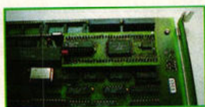
To make this 'naked' Janus20 card spring to life you need a set of TOS 2.06 ROMs (upper left) and a couple of SIMMs RAM cards (left).
