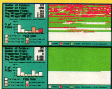
Top: A hard drive partition which has seen some heavy use. The white sections are free space, and the green sections are unfragmented files. Look at how much red there is – these are fragmented files.
