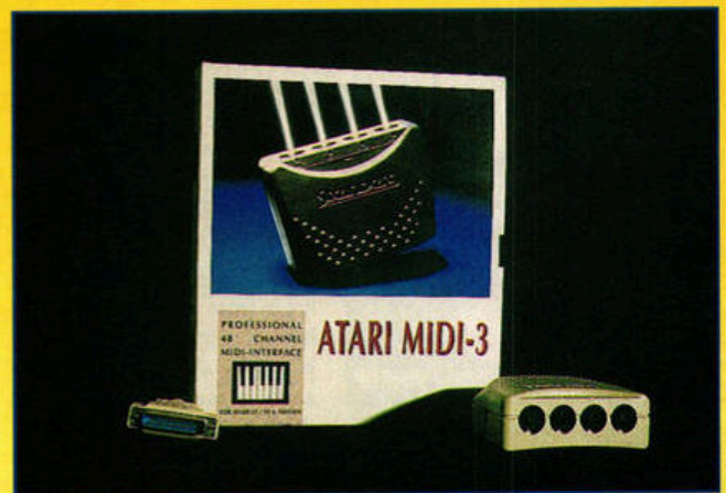
Steinberg's neat MIDI expander not only provides three extra output banks, but also enables you to input MIDI.
