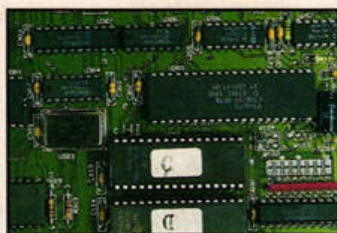
The DMA chip (above the TOS chips) handles intensive data transfers.
