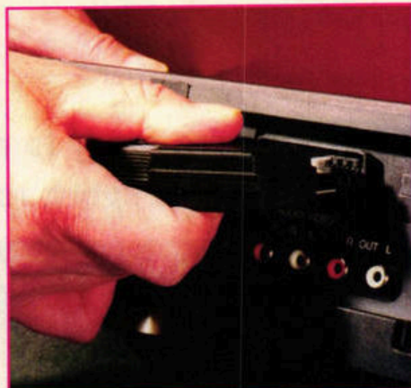
With a SCART plug, one simple connection handles video, audio and the control data needed by your video gear.
