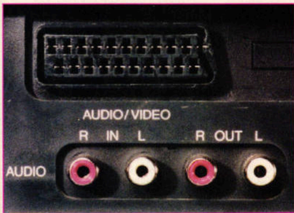
Many video recorders offer both SCART and phono sockets. Use the SCART connector if possible, because it provides a better RGB signal.
